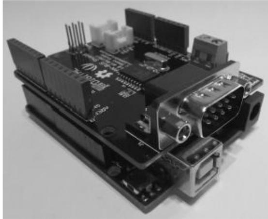
In terms of CAN capabilities, the shield by Seeed Studio provides the same functionality as the one by SK Pang electronics, however, it comes with a much lower price tag, because it does not have any additional components besides the CAN interface.
