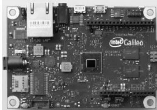
The Intel Galileo is a microcontroller board based on the Intel® Quark SoC X1000 Application Processor, a 32-bit Intel Pentium-class system on a chip. It is designed to be hardware and software pin-compatible with Arduino shields designed for the Uno R3.
