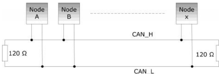
While, for instance, TCP/IP is designed for the transport of large data amounts, CAN is designed for real-time requirements and with its 1 MBit/sec baud rate can easily beat a 100 MBit/sec TCP/IP connection when it comes to short reaction times, timely error detection, quick error recovery and error repair.
