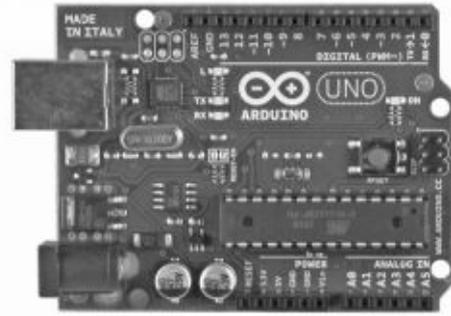
In order to develop and test the sample programs (sketches) as shown in this book, I used the Arduino Uno. The hardware consists of an open-source hardware board, usually designed around an 8-bit Atmel AVR microcontroller with 2 KB RAM (working memory), 32 KB Flash Memory (sketches) and 1 KB EEPROM (non-volatile).
