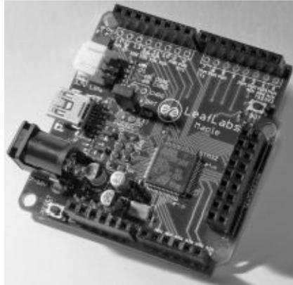
As similar as it may be to the Arduino, the differences are what really make the Maple stand out. It harnesses the power of a 32-bit ARM Cortex-M3 clocked at 72 MHz to push 39 GPIOs, 16 analog pins, 12-bit ADC resolution and 15 PWM pins at 16-bit resolution. In order to make sure you have plenty of programming room to flex that hardware, the Maple also provides 128k Flash and 20KB SRAM. All of this performance is delivered in the same form factor as the Arduino Pro.
