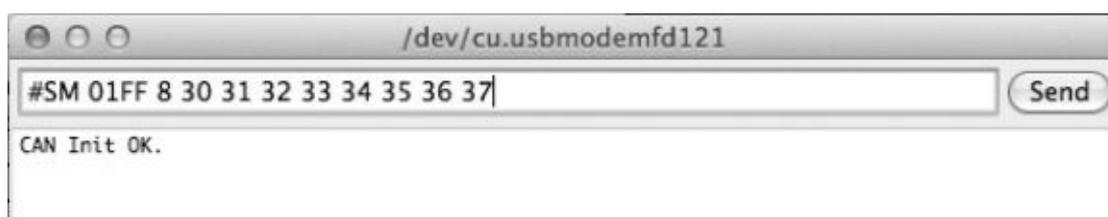
While the basic functionality of sending and receiving CAN messages remains the same, the program size and complexity has, naturally, grown. Most of the code, however, is being used for conversion between hex and ASCII formats (for readability) and some rudimentary syntax check.
