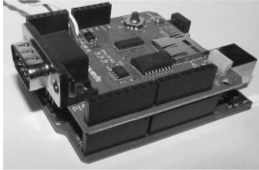
This shield by SK Pang electronics provides the Arduino CAN-Bus capability. As explained previously, it uses the Microchip MCP2515 CAN controller with MCP2551 CAN transceiver. The CAN connection is realized via a standard 9-way sub-D, however the pin assignment for CAN\_H, CAN\_L is not according to standard.
