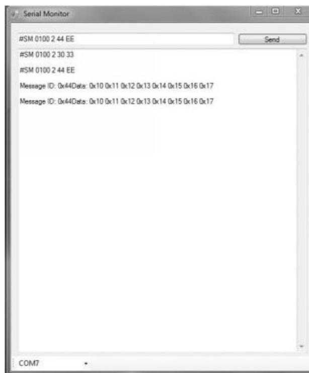
In this case, we sent two CAN Messages with the same ID (0100) but different data. Next, we received two messages through my standard test configuration (i.e. USB-to-CAN gateway with Windows monitoring tool as the second CAN node).
